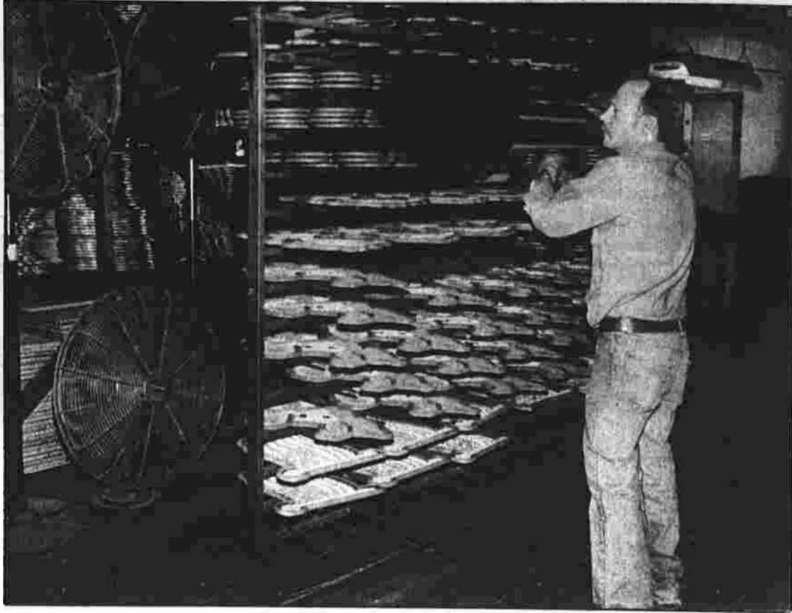
OVEN FRESH - George Nickerson places a rack of plastic molds, that were just melted in a 400-degree oven, in front of cooling fans.
